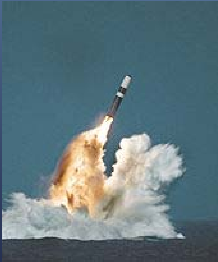
A Trident II missile fires its first stage after an underwater launch
